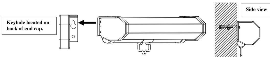
**Note: No hardware is included with this screen for installation.** For wall mounting in to drywall, drywall anchors and screws will suffice to sustain the weight of this screen. For any other type of wall mounting, please consult with your local hardware store to obtain the proper hardware.
