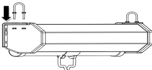
**U-bolts included with Akia Manual series for suspended ceiling installation using chains and S-hooks. (Chains and S-hooks not included)**
