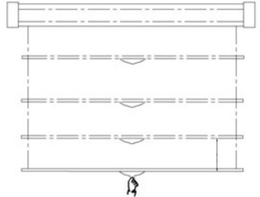
**Attention:** When retracting, always pull the screen down at a 90-degree angle. If ever the screen feels stuck, keep in mind that the screen's mechanism is new and needs to be run up/down a few times to loosen up. If this happens, carefully, with a little force, yank the screen straight down to unlock the mechanism.
