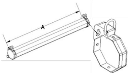
Step 2: Drill a hole for each screw hole on the marked areas. Insert a **dry-wall anchor** into the wall. Then screw the **M5x60 Screw** in each **dry-wall anchor** in leaving about 1/8" of an inch.
