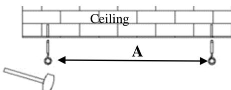
Step 3: Attach the snap link through the eyebolt and connect it to the loop on the screen's end cap.
