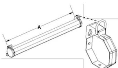
Step 2: Drill a hole on all marked areas and insert the M6.5 eyebolt screw into the hole, then screw up with hammer.
