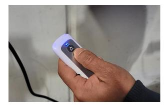
**Step 3.** While holding the STOP button, plug the screen back to the power outlet. (The screen should drop and retract to confirm the sync process)
